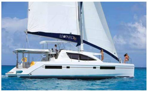
The Leopard 48 features an extremely sporty space-age profile that incorporates several interesting design concepts, including a forward cockpit with an overhead hatch and a raised helm station with a solid hardtop dodger for sun protection. A four-cabin charter version is available as the Moorings 4800.
