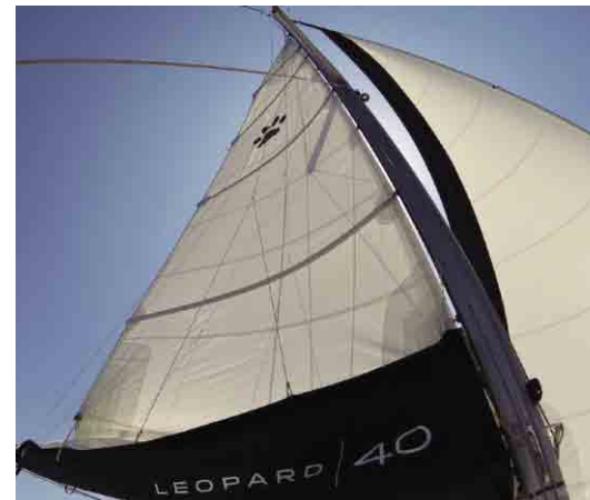
The large roached mainsail is an option worth having on the Leopard 40. Photo Kevin Green
