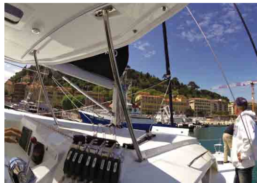
The steering bimini has a useful window on the GRP to view the mainsail. Photo Kevin Green
