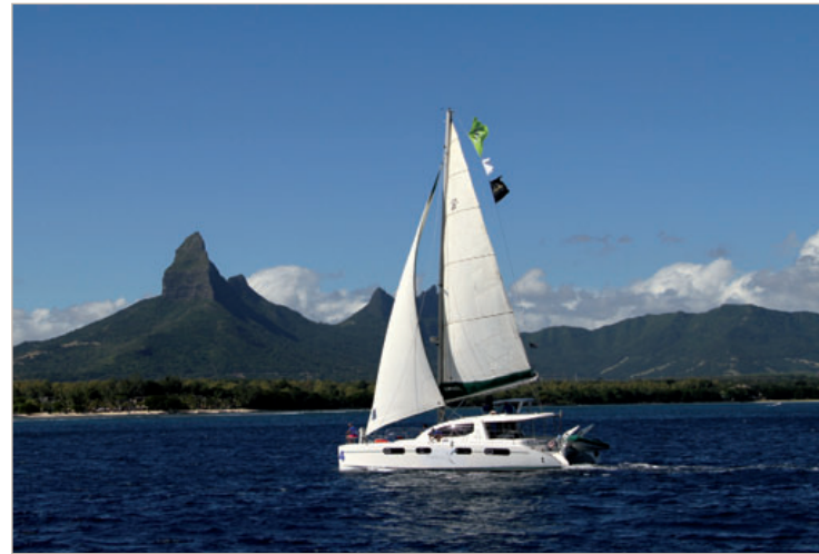
The sail plan is quite generous... The mast is tall; the roach and the genoa's overlap are significant.
