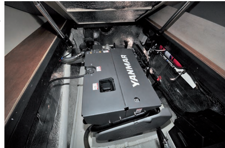
→ The 6-cylinder Yanmar 31 turbo motors develop 260 hp. Opening the engine compartments is easy, thanks to two electric rams
