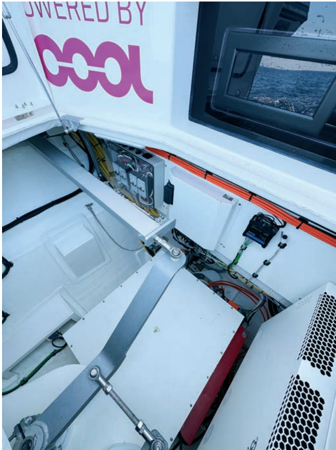
The engine compartment houses the 27-kWh battery and the various components of the Jooool system.
