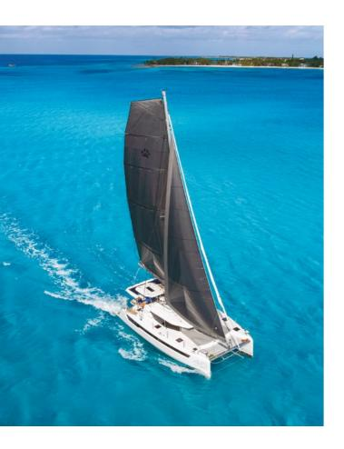
With a taller mast and optional performance Aramid Sport sail rig she has 15% more sail area, including upgraded running rigging for ease of maneuvering, delivering superior performance in all wind conditions and together with stepped hulls, allows for effortless steerage on a well-balanced helm. The helm layout is simple and functional in layout for one handed sailing.
