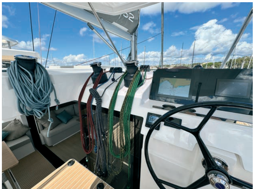
The helm station has been designed for single-handed sailing. It offers good protection, and all the halyards are within easy reach.
