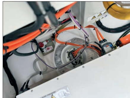
The electric propulsion system is housed in the same location as the diesel engines and includes two 25-kW pods.
