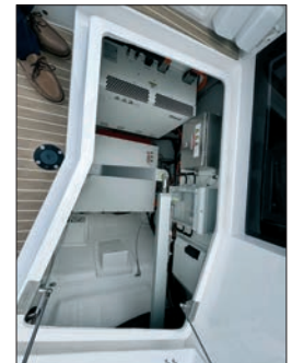
The electric propulsion system is housed in the same location as the diesel engines and includes two 25-kW pods.
