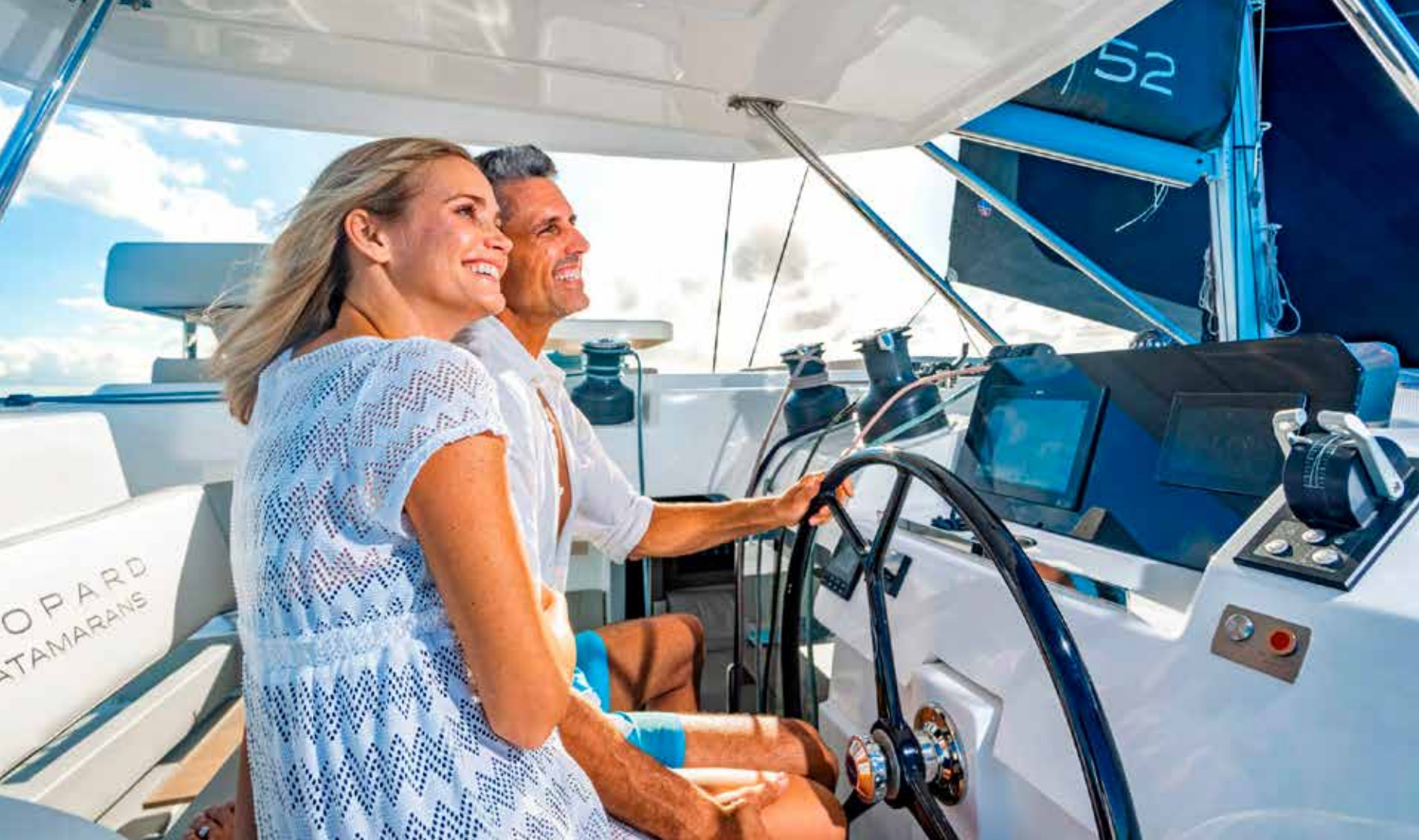
The Leopard 52 retains the brand's semi-raised helm station, which allows vision of much of the exterior, including below to the aft cockpit
