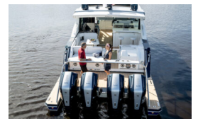
Mercury 7.6l V12 600hp Verado – the largest outboard engine
